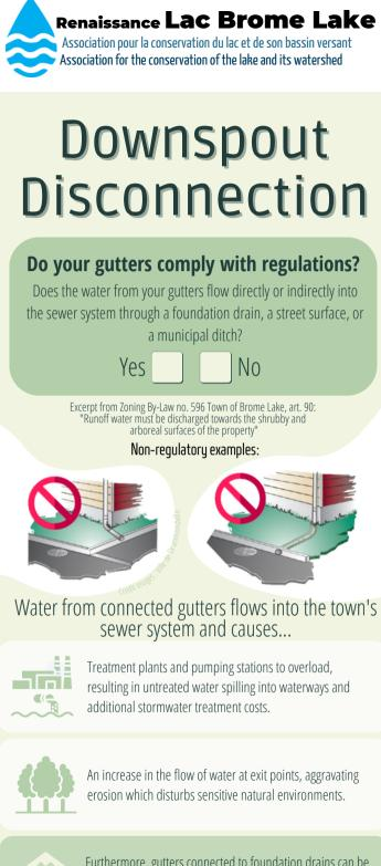
Furthermore, gutters connected to foundation drains can be overburdened causing backflows in basements that can seriously damage a house's fondations.
